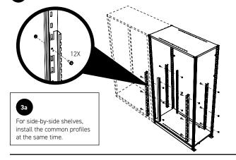
It is recommended to install the rear crosspieces or the rear panels after the mounting profiles have been installed.
